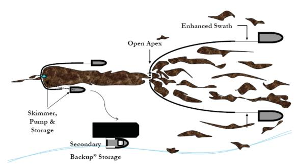
Scattered oil is "caught" by two VOO and collected at the apex of the towed sea boom. The oil moves thought a "gate" at that apex, forming a larger stream of oil which moves into the boom of the skimming vessel. Operations are paced at >1. A recovered oil barge stationed nearby to minimize time taken to offload recovered oil.
