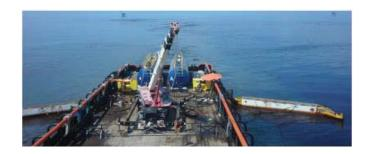
This is a depiction of the same operation as above but using KOSEQ Arms. In this configuration, the collecting boom speed dictates the operational pace at  $\geq 1$  knot to minimize entrainment of the oil.
