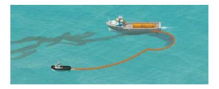
Through the use of an additional VOO, and using extended sea boom, the swath of the VOSS is increased therefore maximizing the oil-to-skimmer encounter rate. Skimming pace is < 1 knot.
